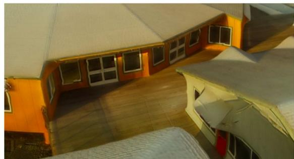
3D models are improved by including oblique images. Image Source: [www.dronedeploy.com](http://www.dronedeploy.com)
