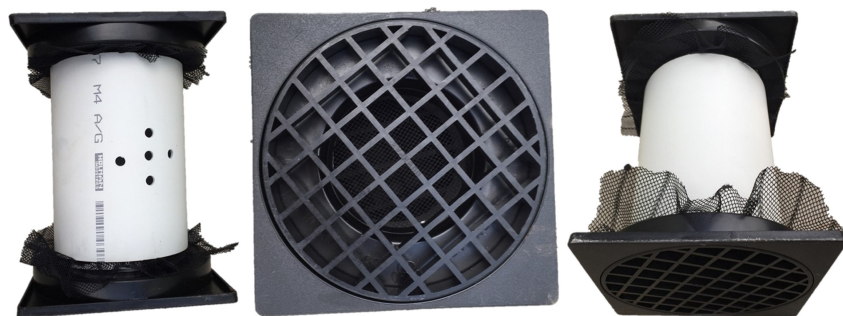
FIGURE 3 Tube used for live frog scent training preventing contact between frog and dog while allowing scent permeation. Consisting of 100 mm section of PVC tube approximately 15 cm long, with each end capped with perforated drainage gutter and fly mesh.
