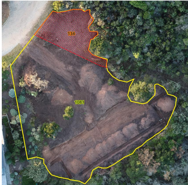
Figure 2: Excessive bush clearing by contractors. The area in yellow shows the full extent of the vegetation cleared for the building. The area in red represents excess clearing which was not part of the landowner's property. Area in metres squared
